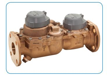
Rotor and disc movements are transmitted by magnetic drive couplings to individual register odometers. The direct magnetic drive provides a positive, reliable and dependable register coupling for straight-reading or remote reading options. The self-lubricating thermoplastic register gearing is designed to minimize friction and provide long life.
